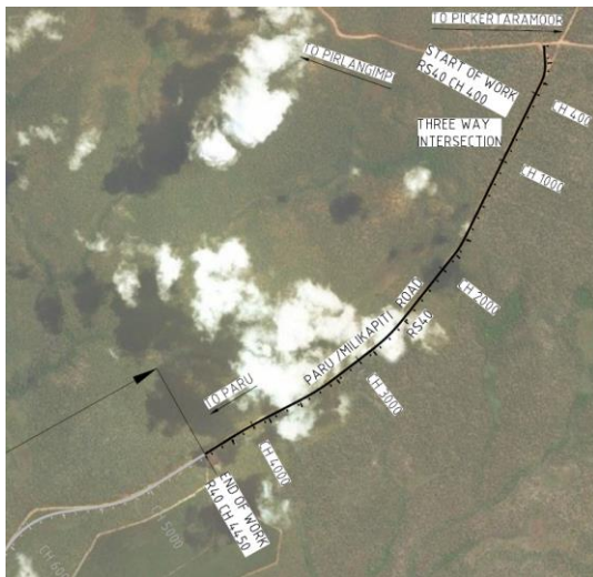
Location: Melville Island - upgrade and seal Paru Road between chainage 0.40km and 4.45km
