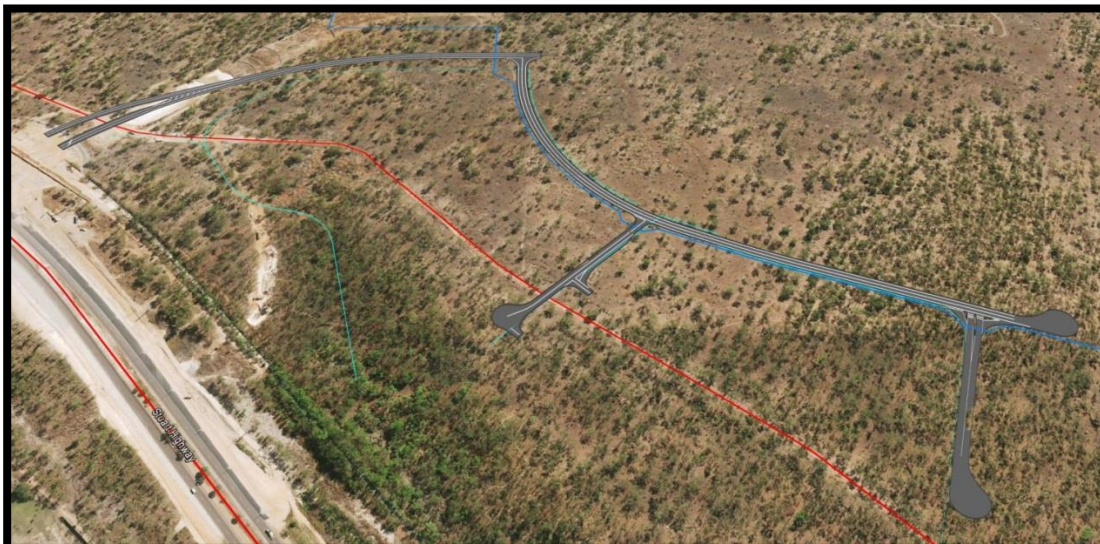
Concept: Glyde Point Road, Holtze Collector Road and PRH Access Roads (also indicating Water main (blue) and Drains (light blue))
