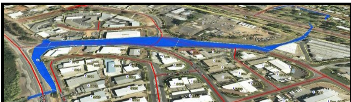
Concept: Ludmilla Creek Catchment Flood Mitigation - proposed Dwyer Park Berm and Associated Drainage
