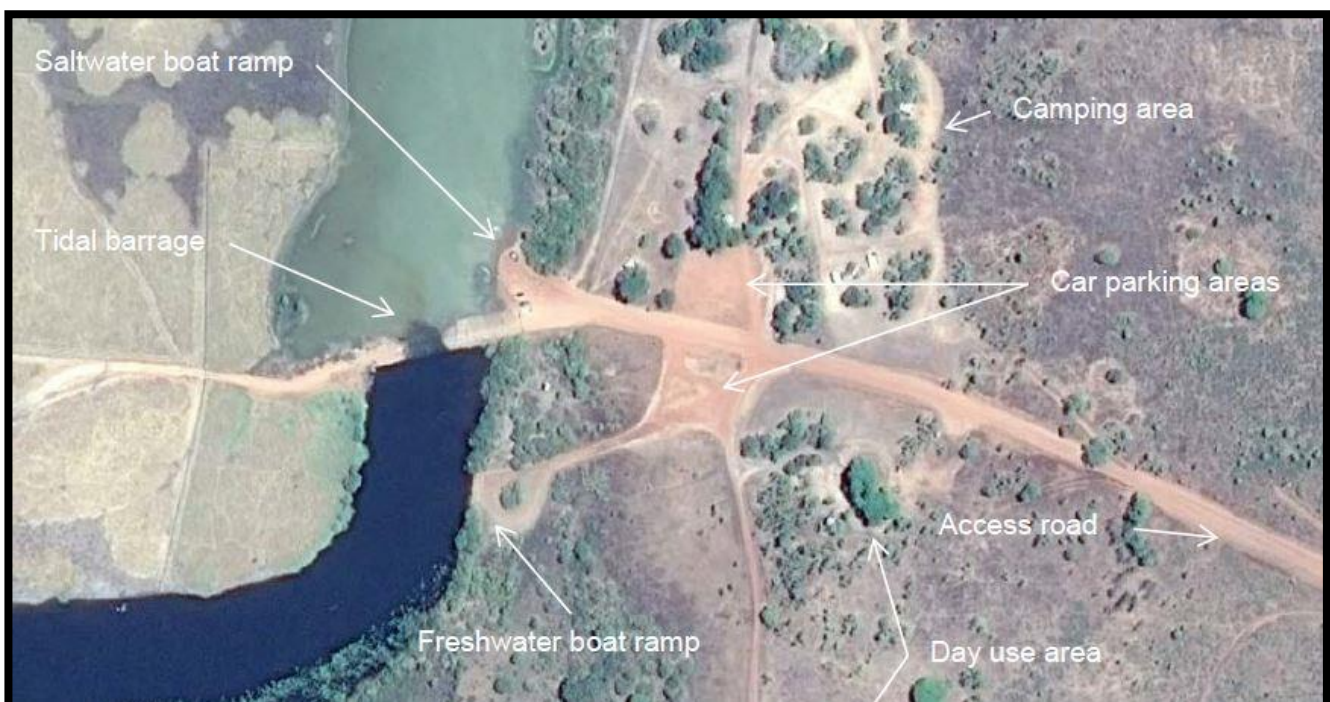
Aerial Photo: Mary River - Shady Camp - 50-metre extension to the boat ramp and sealed parking with 60 marked car and trailer bays
