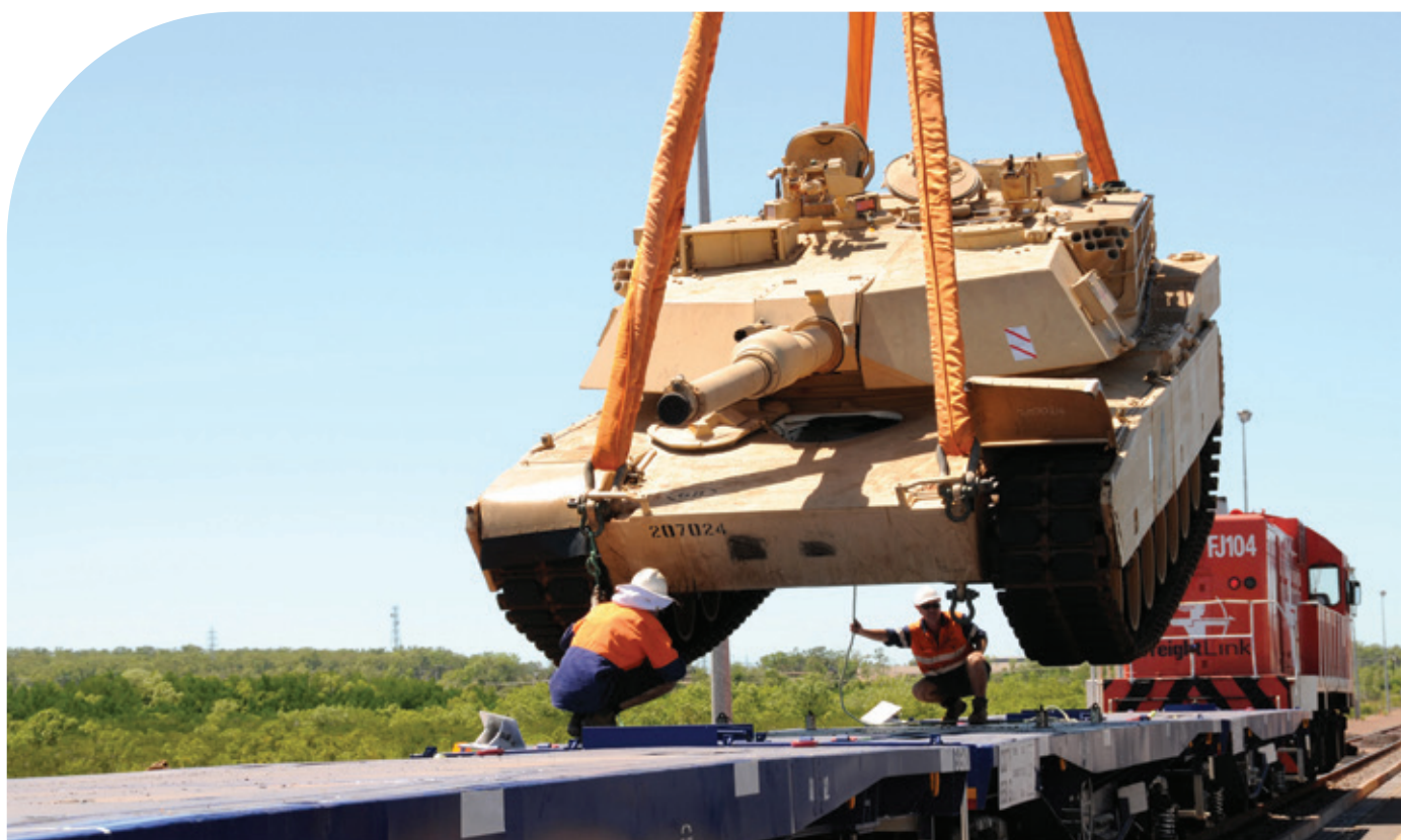
Above: 60,000 kilograms of armour touches down onto the purpose-built rolling stock during loading trials. Credit: Department of Defence. © Commonwealth of Australia, Department of Defence.
