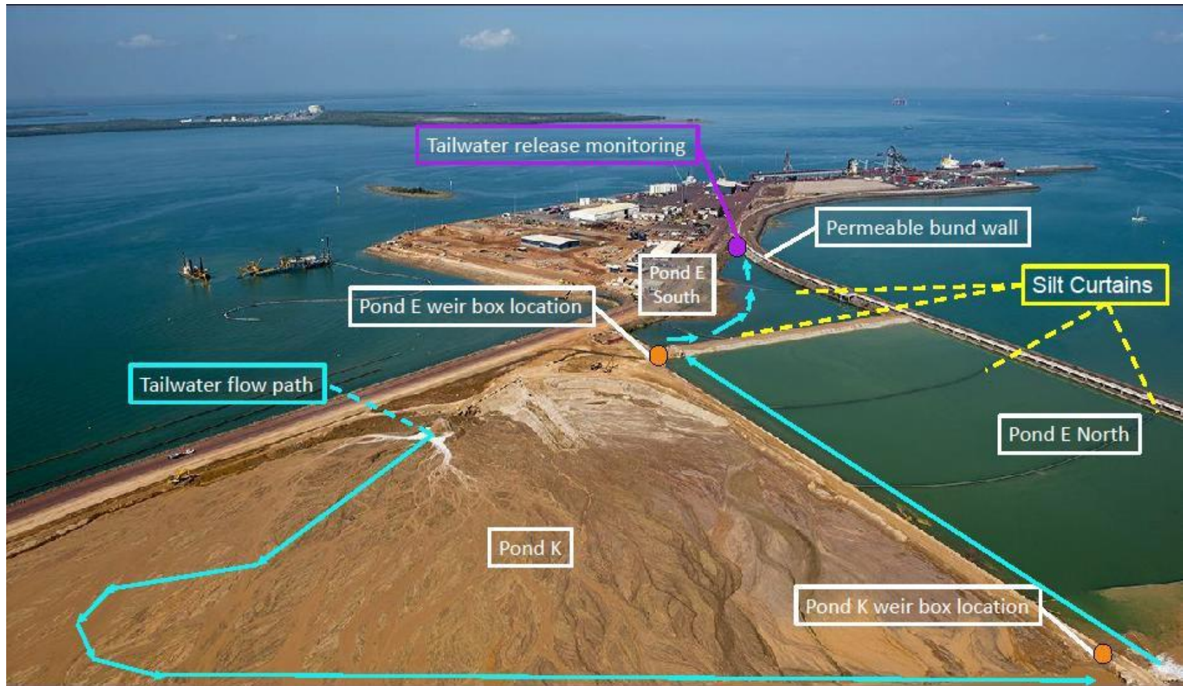
Figure 9 Indicative settling pond configuration
