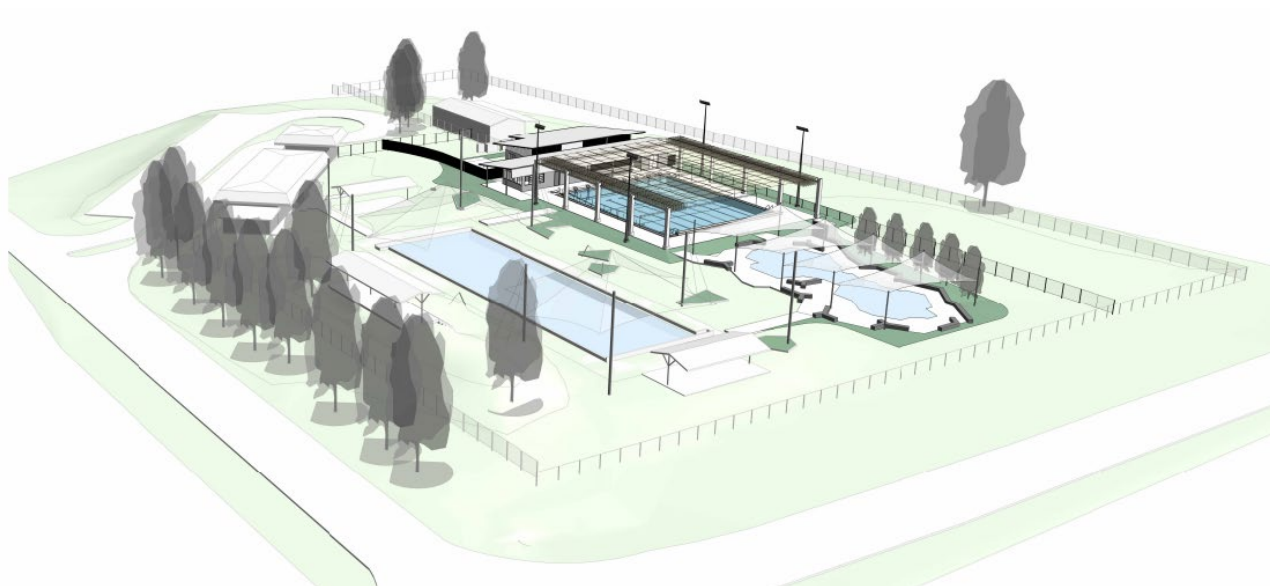
Katherine Aquatic Centre upgrade – new pools, pumps and plant room, rectification of existing pool and change facility Image provided courtesy of Katherine Town Council, Sitzler and Liquid Blu
