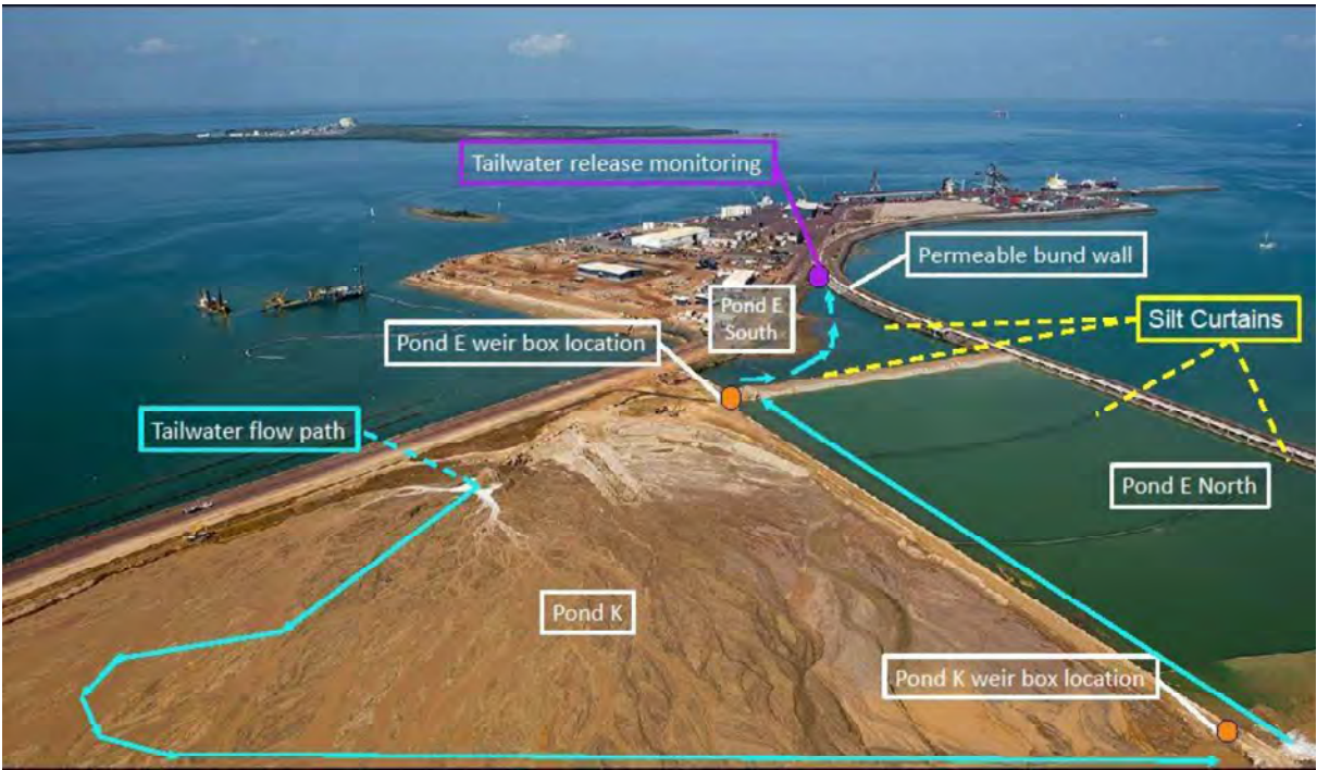
Figure 9 Indicative settling pond configuration
